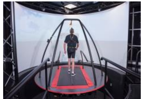
Figure 1: CAREN system. The self-paced treadmill (outlined in red) in front of the projection screen allows the individual to be immersed in an activity or scene.
